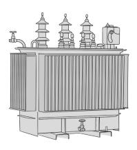
Oil filled transformers have long been a cornerstone of electrical power distribution, using mineral oil or ester fluid as both an insulating and heat transfer medium.
