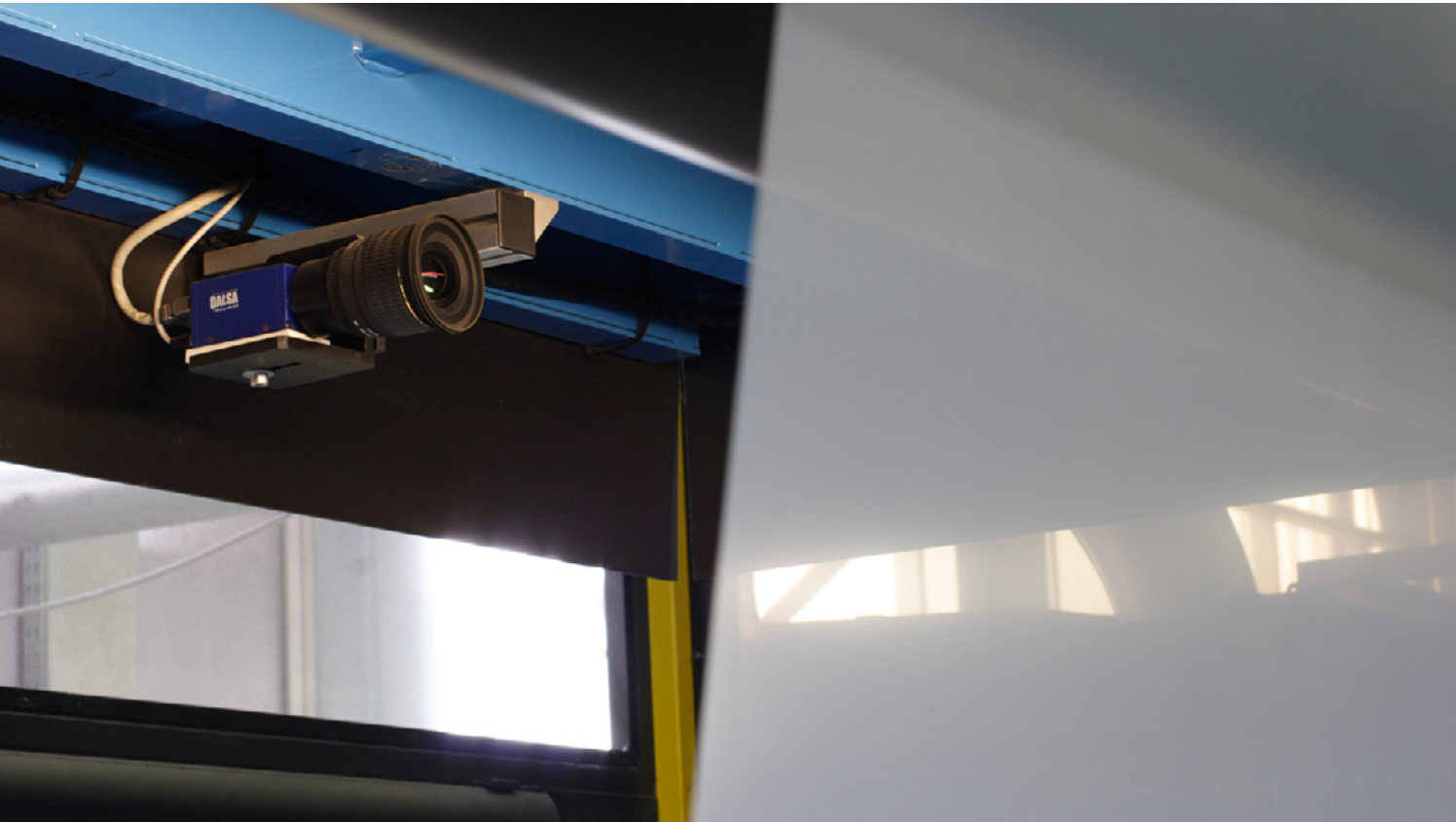
In-line quality control via camera
