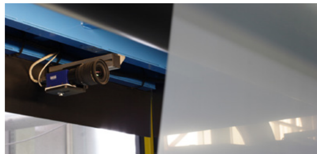
In-line quality control via camera
