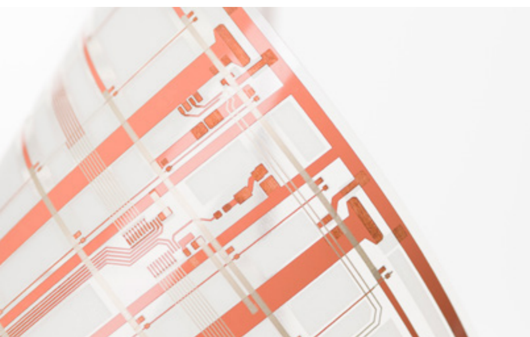
Film printed with a copper circuit
