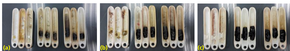
Figure 4-8: Pictures of char residues (from left to right PPE, TPT, KPK; top down 300 °C, 400 °C, 500 °C)
